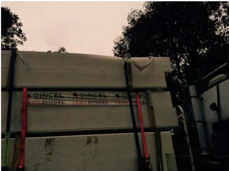
***Please note that at no time will Dincel Construction System allow a vehicle to be dispatched as shown in the above pictures.*** If a truck arrives on site that has not been loaded and restrained correctly we recommend you hold your transport provider responsible for the potential damages.
